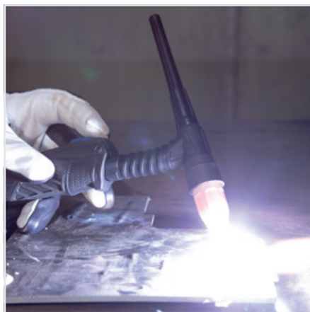
(2) Press the torch switch and the arc will ignite across the gap between the tungsten and work piece. Hold even distance of about 2mm gap between the tungsten and work piece to maintain the arc.
