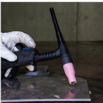
(1) Lay the outside edge of the Gas Cup on the work piece with the Tungsten Electrode 1- 3mm from the work piece.
